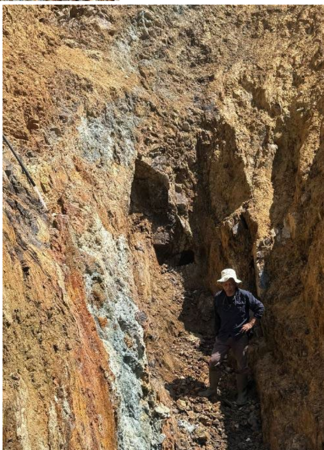
Figure A2 – Another small mine working in the north of the EL02 license. Looking NW. Note on left side of trench, sulfide mineralization (gray color) in hangingwall of fault surface.
